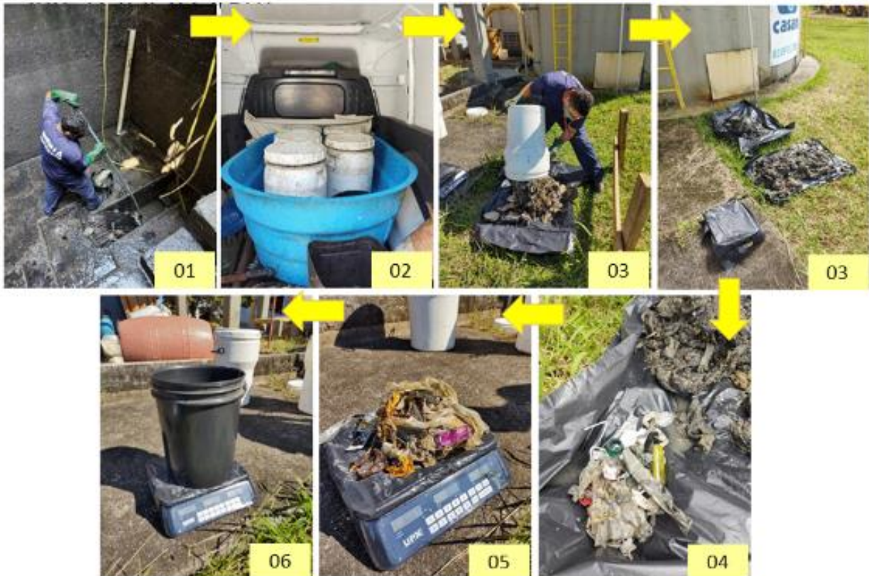
Figure 3. Example of the main steps of the gravimetric study (in this case, image 01 shows the removal of waste from the grid in SPS HU/Trindade).
