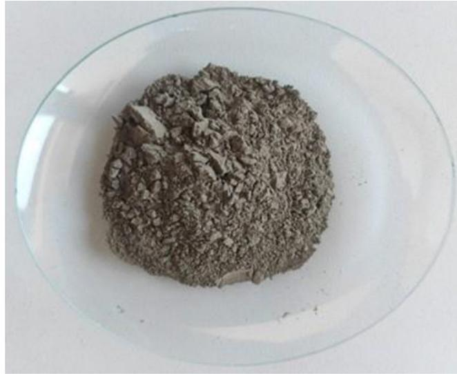
The samples were homogenized in sieves with a mesh size of 0.30 mm (ABNT, 2024). X-ray fluorescence analysis was used to quantify the main oxides present in basaltic rock-hematite, alumina, calcium oxide, magnesium, potassium, phosphorus, and manganese-, which was performed at the laboratory SGS Geosol, located in Belo Horizonte, Minas Gerais, Brazil.
