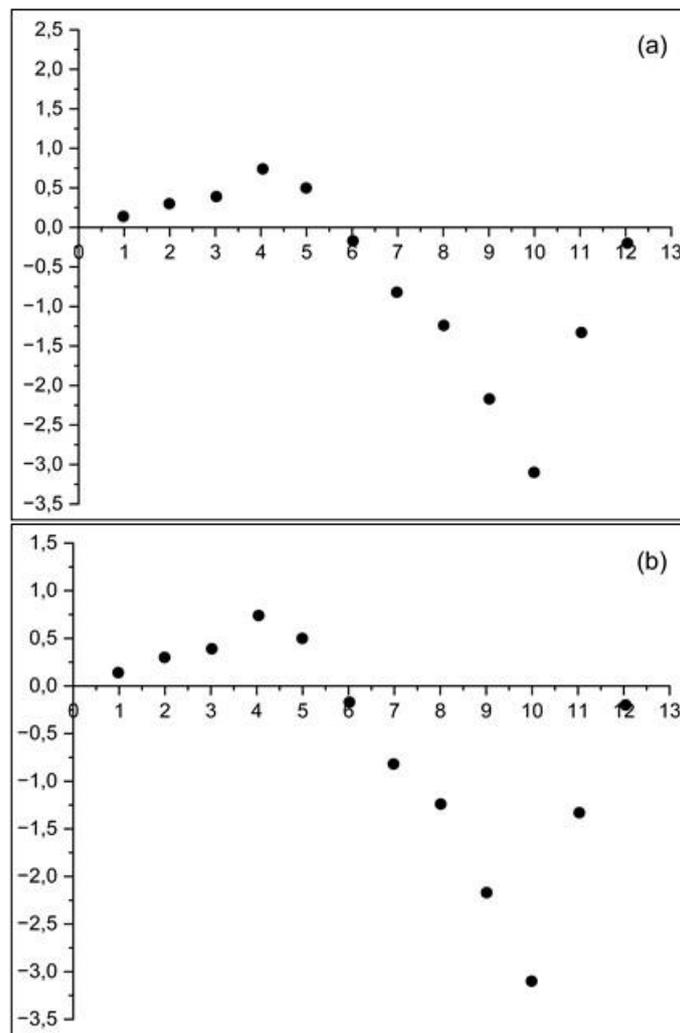
For the pH range considered, the values of the adsorbents'  $\text{pH}_{\text{ZPC}}$  were determined by the intersection points of the respective curves with the x-axis. Thus, the values are 6.5 and 5.5 for basaltic remineralizer and nano-hematite, respectively.
