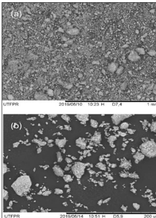
Its morphology can be described as amorphous with dispersed particles with heterogeneous clusters. In their research, Shrimali *et al.* (2016) found, with the SEM images, smooth and uniform surfaces of iron oxide particles. In contrast, Moreira *et al.* (2017) found uniform spherical and monodispersed nanoparticles for iron oxide, indicating that the process of obtaining hematite can significantly change its surface morphology.
