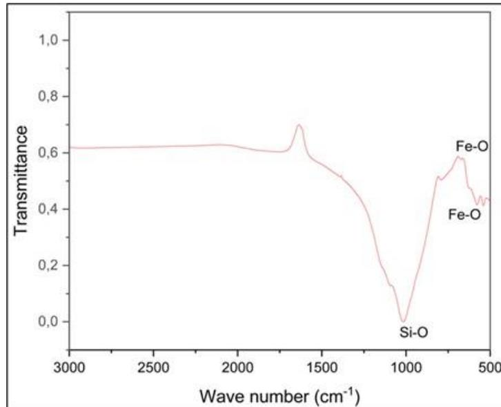
**Figure 4.** Infrared spectroscopy with Fourier transform (FTIR) for samples of hematite nanoparticles
